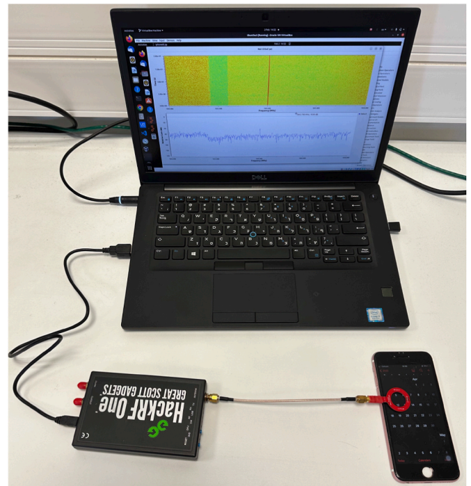
Fig. 1. Acquisition of electromagnetic (EM) traces while carrying out various software activities on the iPhone using the HackRF One SDR connected with H-loop near-field antenna and controlled by GNU Radio Companion.
